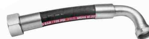
DISCHARGE HOSE MAX. WORKING PRESSURE : 50 BAR LENGTH : 500 mm Aprox ELBOW INLET : 1-7/8" / 48 mm OUTLET : 2" / 51 mm SLAVE CONNECTION : 1/8" / 10 mm
