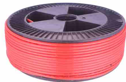
HEAT SENSING TUBE (HST) COLOUR : Red DIMENSION : 6×4mm(ODxID) OPERATING PRESSURE : 15Bar BURST TEMP : 130°C-141°C
