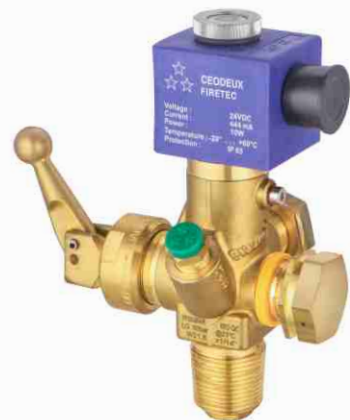
GAS DISCHARGE VALVE G TYPE M.O.C : Forged Brass ACTUATOR CONNECTION : Inbuilt 24V DC DISCHARGE CONNECTION : 3/4" / 20 mm CYLINDER CONNECTION : 1" / 25 mm
