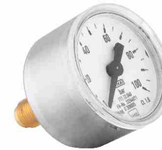
PRESSURE GAUGE TYPE : Spring Tube Manometer RANGE : 0 to 100 BAR CONNECTION : 1/8" NPT
